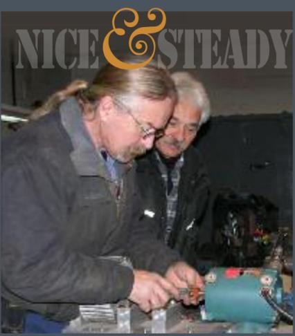
Geoff Greene, left, a 25 year veteran of Longo's Field Service group, and Wayne Forte, right, Vibration Analysis Technician, are shown setting up one of Longo's unique training and demonstration pieces. When completed, the unit will demonstrate the weakness in placing a fan at the end of an unsupported shaft.
