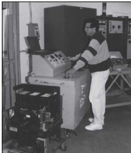
Injection current testing for comparison with manufacturer's trip characteristics
