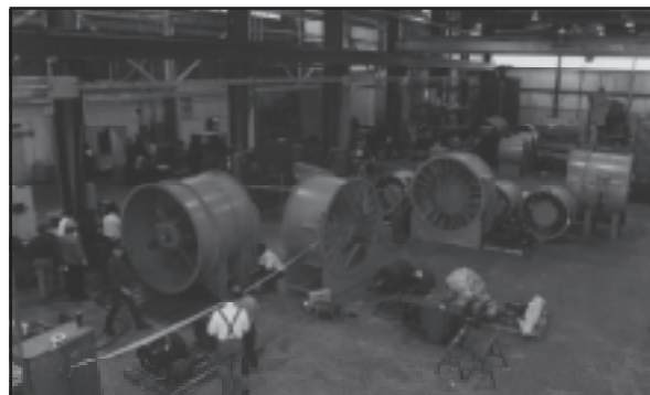
A 350 HP fan under customer witnessed full load test. Our test bed is a necessary requirement for securing the unit and isolating extraneous vibrations from the unit on test.
