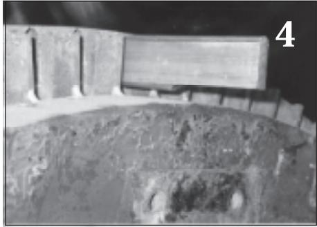
Diecast rotors can not be repaired when defective. They must be either recast or converted to fabricated rotor construction. Recasting requires removal of the original material by chemical means, then recasting with an equivalent conductivity material.
