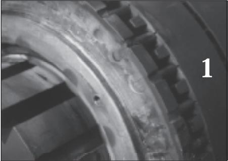
Rebrazing requires controlled conditions to be certain that thermal and mechanical stresses are minimized, and thereafter relieved. Repaired joint integrity must be verified after brazing, using nondestructive techniques such as ultrasonic testing. At best, rebrazing is a “fix”, not a cure. The inherent weaknesses that led to the cracking have not been removed.
