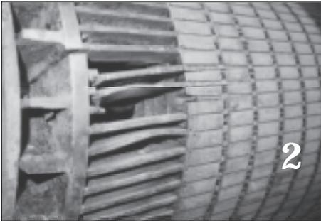
a defect that will require rebarring. Following this, rotor bar and endring materials are selected so as to provide the optimum rotor for the intended use. The same section of the defective rotor of **Photo 2** is shown in **Photo 3**, after rebarring. Construction details, such
