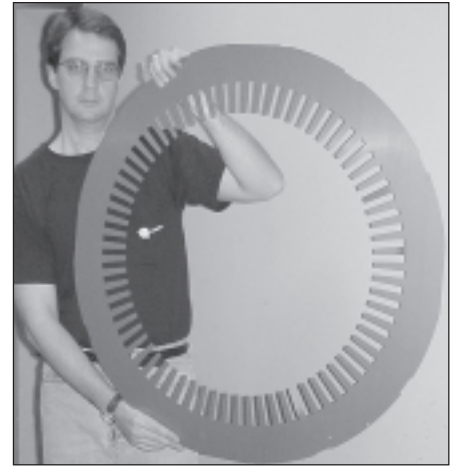
A single punching, which is one of several hundred stacked, then compressed to accommodate the windings which make the magnetics when energized.
