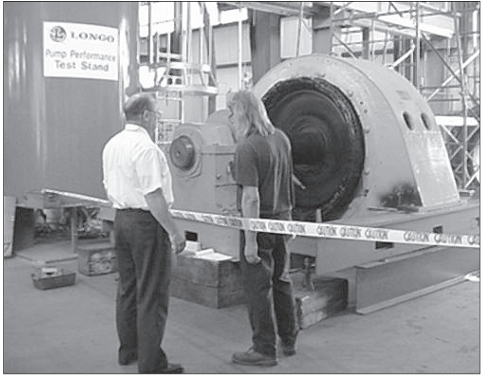
Photo 1 - A very large synchronous motor being run-tested.
