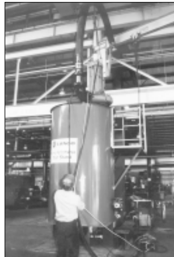
Pump performance testing & documentation . . . an integral part of a quality rebuild.
