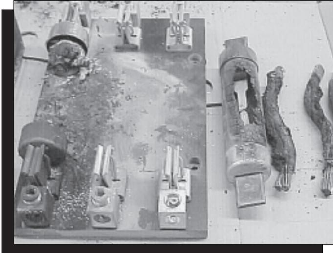
This is a digital image of an actual failure of a 480 volt fused disconnect panel.
