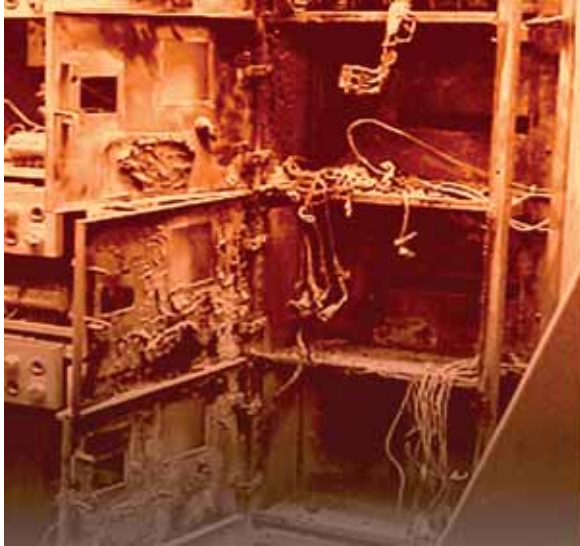
Above; faulty switchgear explosion. The Longo Servicenter is set up to handle switchgear, circuit breakers and transformer service, as well as the "plug and play" replacement units.
