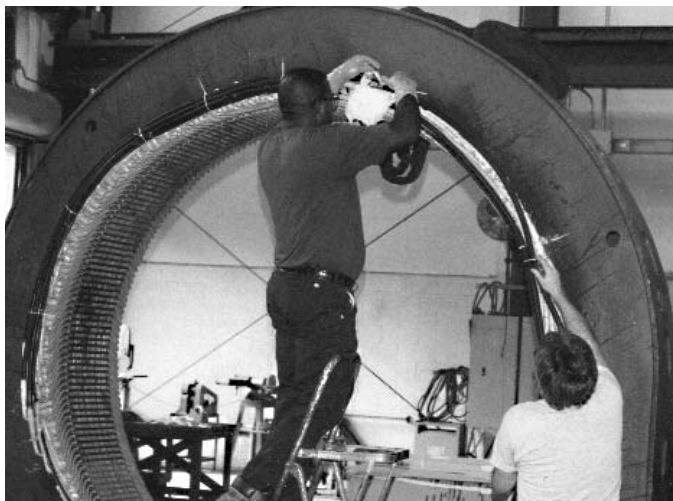
Relamination completed, new windings installed, the motor leads are installed.
