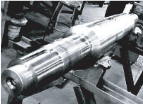
On Wednesday, June 22, 2004 a condensate pump motor in Philadelphia snapped a shaft. Ordinarily that isn't big news. Pull the motor and replace it with a spare. Simple. Only this was a vertical 900 hp/4000 volt motor weighing in at 38,000 lbs; so when the shaft broke it got very ugly, very quickly. The rotor dropped, hit the stator, and basically tore up the motor.
