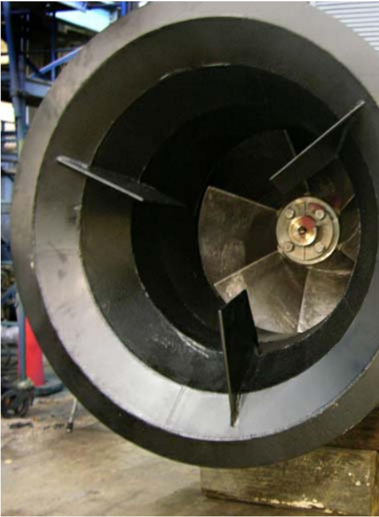
*The finished pump is ready to be loaded onto the Longo flat bed and delivered to the cusomter. The final turn around time was actually 13 days which included unexpected time for re-machining the bore of the center casing.*
