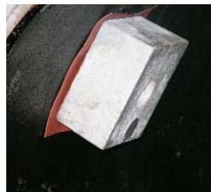
*Left: The magnesium anode is probably one of the most "low tech" solutions to corrosion still in use today.*
