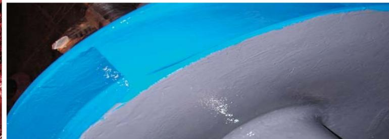
This volute, part of a 20,000 GPM, 500 hp pump, took quite a beating from waste water laced with sodium hypochlorite. Both the outer edge and the inner surfaces were savaged in spots. The first reaction would be to get a new volute, but that has a few drawbacks. It can take up to 20 weeks and they are very expensive.
