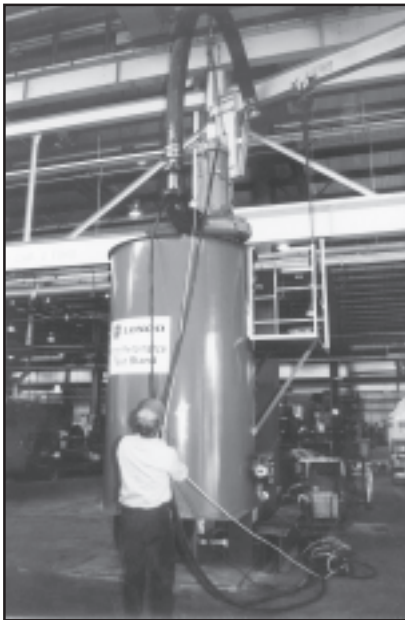
Test tank is 10 ft. high, 6 ft. in diameter
