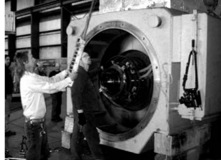
*Left: Thanks again to the 100 ton crane, the removal of the rotor from this mammoth motor was done with the ease of doing a 500 hp motor back in the shop.*
