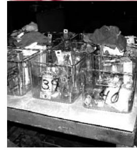
With balance such a critical aspect of the project, it is essential that all the components, the diodes, fuses and even down to the washers are kept together. Each "family" of components is marked with their position number. To take it one step further, they are all kept in their own containers through out the process. Although almost mundane, the amount of touches on this unit is extremely high when you extrapolate the numbers. This is where a professional approach is essential to ensure each and every item removed and replaced accurately.
