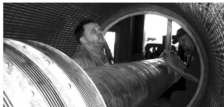
Below: Hi-tech gives way to hands-on and eyes-on in order to make sure that there is nothing left from the exploding cast aluminum fan blade.
