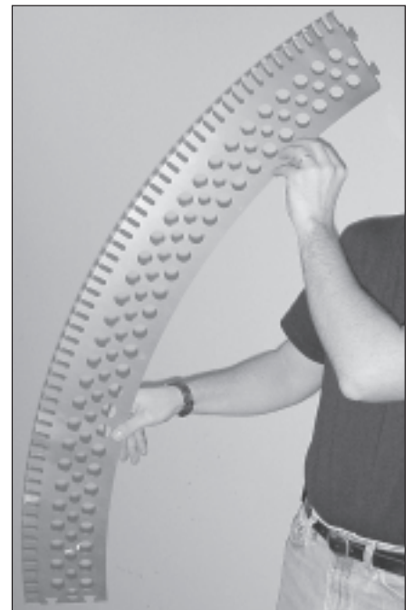
A new section of lamination for a very large rotor. Notice the circular holes, which provide cooling for the iron.
