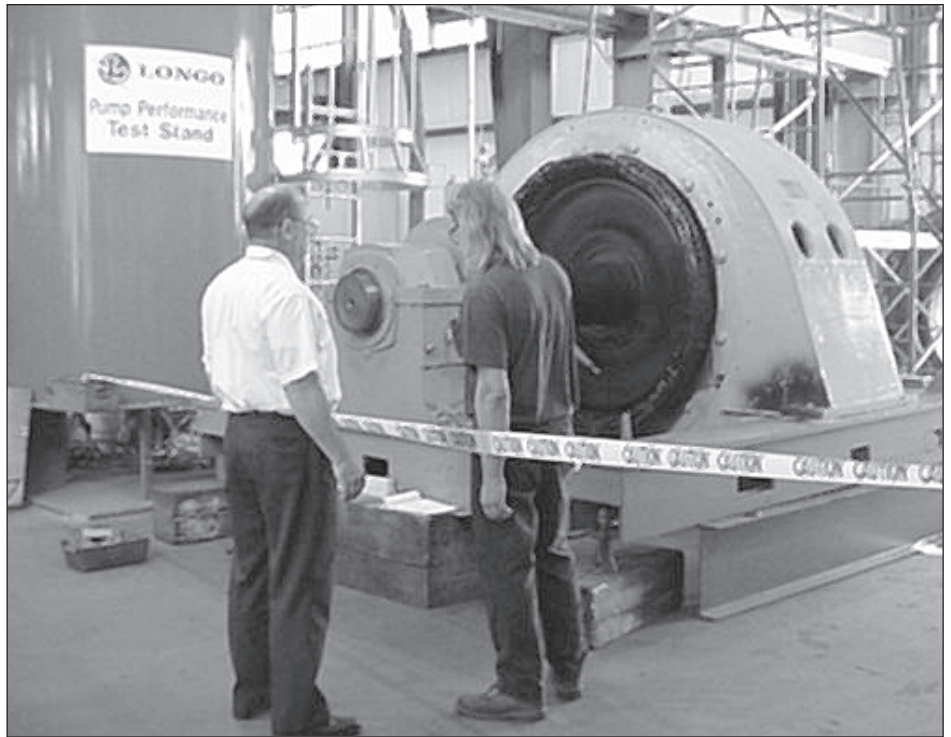
Photo 1 - A very large synchronous motor being run-tested.
