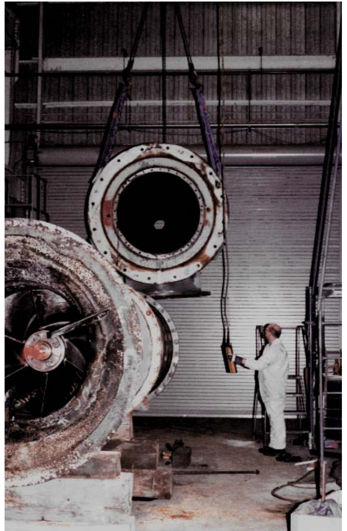
Above: You see the size of the pump and its sections. The right equipment, a 25 ton crane, and correct rigging makes the disassembly of the giant pump seem like childs play..
