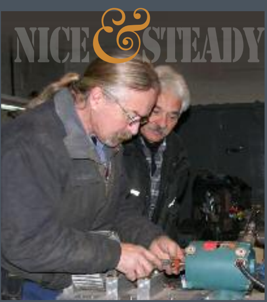
Geoff Greene, left, a 25 year veteran of Longo's Field Service group, and Wayne Forte, right, Vibration Analysis Technician, are shown setting up one of Longo's unique training and demonstration pieces. When completed, the unit will demonstrate the weakness in placing a fan at the end of an unsupported shaft.
