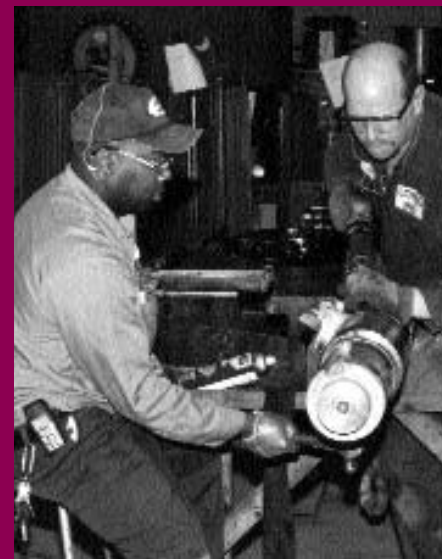
The main shaft of the pump was examined, worn protective sleeves removed and the shaft was checked for balance and straightness.
